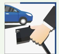
Plug the charging cable into your vehicle and select "Start Charging" on your device screen and press the "Start" button on the charger
